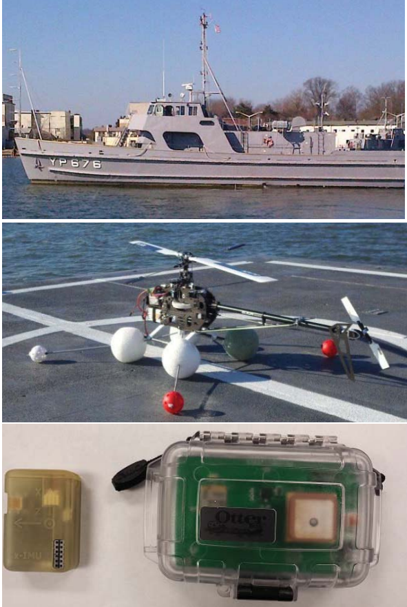
Fig. 1: Experimental Setup: (a) YP676 training vessel (Top), (b) Instrumented RC Helicopter on Deck (Middle), (c) IMU and GPS sensor (Bottom)
