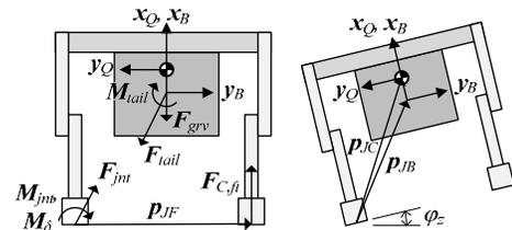
Figure 4. Roll-angle model free-body diagram.
