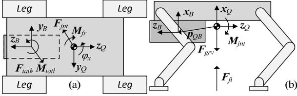
Figure 3. Yaw-angle model free-body diagram: (a) top view, (b) side view. The tail is not shown as its loading effect are captured by  $F_{tail}$  and  $M_{tail}$  and its mass and inertia are captured in  $m$  and  $I$ .
