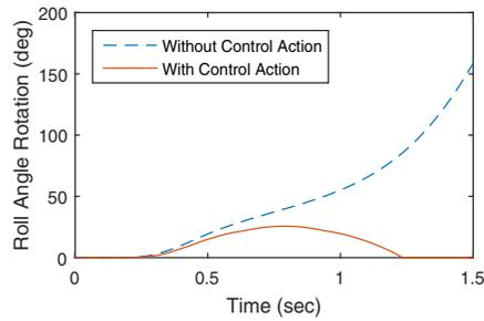
Figure 8. Effect of roll-angle control action.
