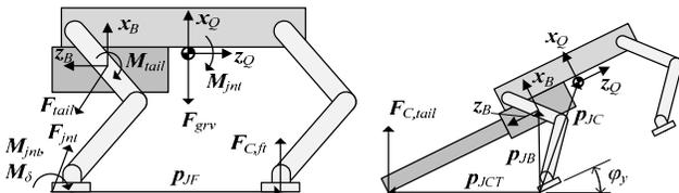
Figure 5. Pitch-angle model free-body diagram.
