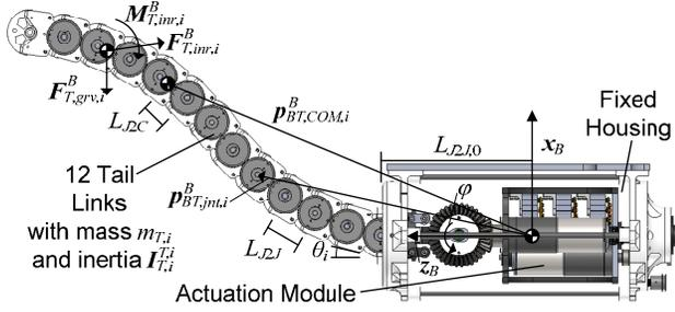
Figure 2. R3RT with relevant kinematic and loading parameters labeled. segment, and the cables are routed along cylindrical surfaces to ensure equal extension/retraction of the cable pair. These cable pairs are connected to spools actuated by a gearmotor through a bevel gear transmission.
