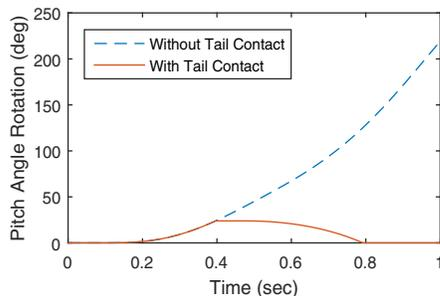
Figure 9. Pitch-angle rotation stabilization due to tail presence.
