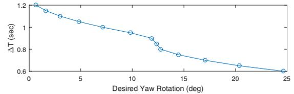
Figure 6. Yaw-angle  $\Delta T$  calculating based on desired  $\varphi_x$ .
