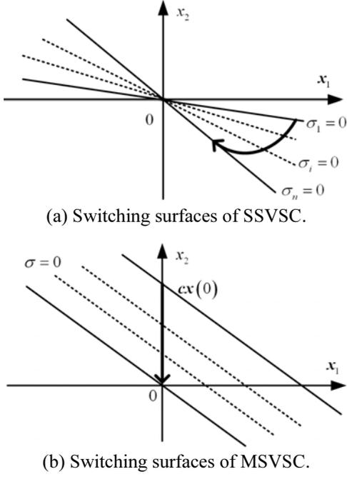
Fig. 4. Switching surfaces in phase plane.
